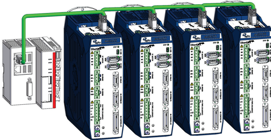
Figure 3. EtherCAT network with AGD155-EC drives
