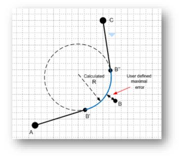
Note that the resulted CNC trajectory does not pass through the original point B and that the original linear segment AB is shortened to be AB' and similarly BC is shortened to be B"C. All the required calculations are automatically performed internally by the controller.
