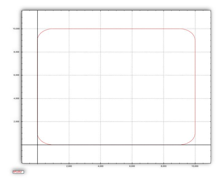
This CNC motion uses axes A and B as members. The graph shows BPosRef (position reference of axis B) as a function of APosRef (position reference of axis A). The absolute start point of the motion is:
