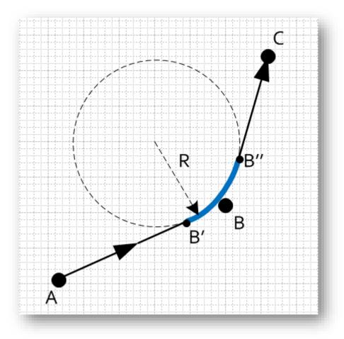
The R (radius of the corner) is calculated based on the following parameters (set using the Set Corner Parameters segment): CornerRadiusMethod and CornerRadiusOrError. If CornerRadiusMethod is 0, then the corner radius is directly the value of CornerRadiusOrError. If CornerRadiusMethod is 1, the radius is calculated so that the maximal error imposed by the corner will be equal to: CornerRadiusOrError, as shown in the following picture:
