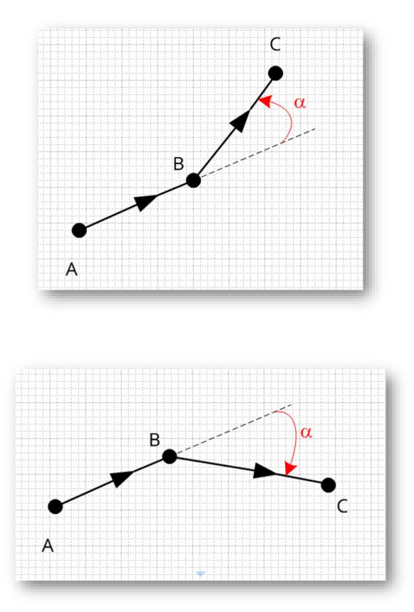
6. Two types of corners are supported: ARC (round corner) and Continuous Acceleration corner. The type of the corner is defined by the last pushed (executed) "Set Corner Parameters" segment.
