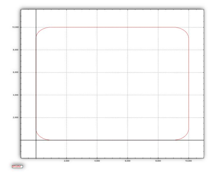
The CNC motion consists of a sequence of motion segments. The CNC profiler in the controller calculates the CNC motion along the CNC path, using parameters provided by the user for the vector acceleration, deceleration, speed and end speed. Once the desired motion along the CNC path is calculated, the relevant motion per each involved axis is derived from this desired vector motion.
